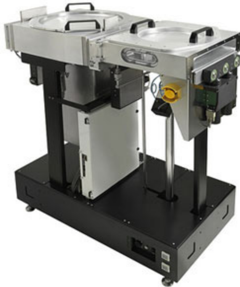
A four-chambered cluster tool can be created using two of the Crossing Automation loadlocks.
